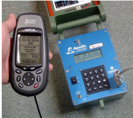
Example of a Connected GPS to an Apollo Counter
